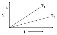
V-I graph for a metallic wire at two different temperatures  $T_1$  and  $T_2$  is as shown in the figure. Which of the two temperatures is higher and why?
