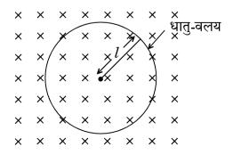
A metallic rod of length 'l' is rotated with a frequency 'v', with one end hinged at the centre and the other end at the circumference of a circular metallic ring, about an axis passing through the centre and perpendicular to the plane of the ring. A constant and uniform magnetic field B parallel to the axis is present everywhere.
