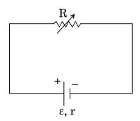
A variable resistor R is connected across a cell of emf  $\epsilon$  and internal resistance r as shown in the figure. Draw a plot showing the variation of (i) terminal voltage V and (ii) the current I, as a function of R.
