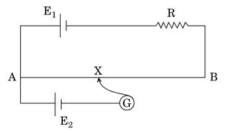
In the circuit diagram shown, AB is a uniform wire of resistance 15  $\Omega$  and length 1 m. It is connected to a cell  $E_1$  of emf 2 V and negligible internal resistance and a resistance R. The balance point with another cell  $E_2$  of emf 75 mV is found at 30 cm from end A. Calculate the value of the resistance R.
