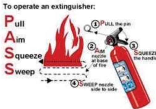
Fig. 3.3.10. Method of operating Fire extinguisher
