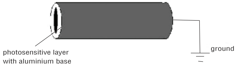
Fig. 13 Photosensitive Drum with aluminium base
