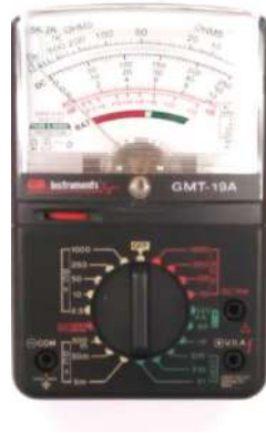
Fig. 5. Although replaced with DMM in many hand-held operations, analog multimeter or VOM is still around
