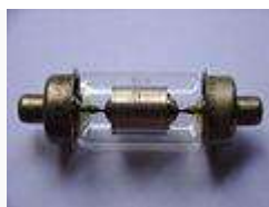
Vacuum capacitor with uranium glass encapsulation
