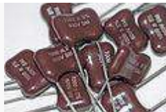
Some 1nF × 500VDC rated silver mica capacitors
