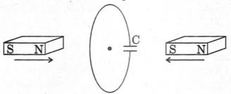
Predict the polarity of the capacitor in the situation described in the figure.
