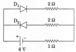
Assuming that the two diodes  $D_1$  and  $D_2$  used in the electric circuit shown in the figure are ideal, find out the value of the current flowing through  $1\ \Omega$  resistor.
