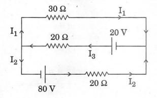
Use Kirchhoff's rules to determine the value of the current  $I_1$  flowing in the circuit shown in the figure.
